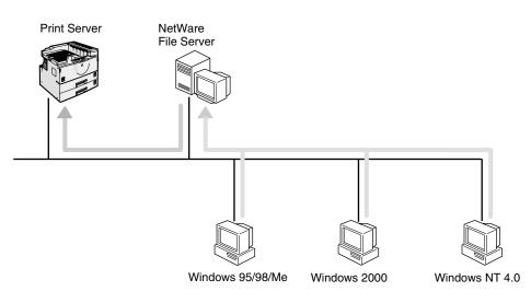
The actual procedures for configuring the printer differ depending on the version of NetWare.
